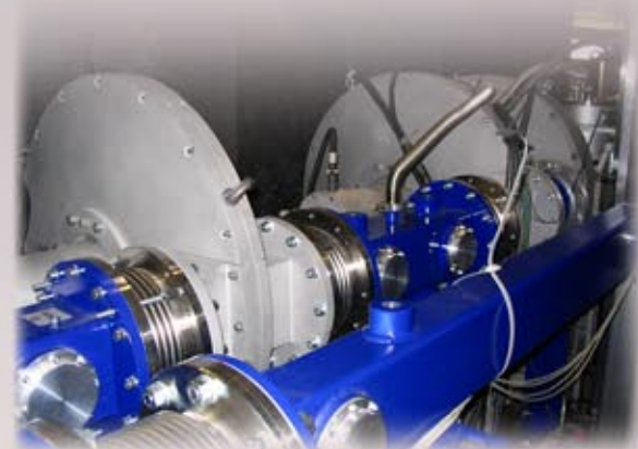
Chopper System driven by Magnetic Levitated Bearing
