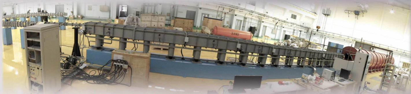
Installed collimator unit of the CARR ICCAS SANS instrument
